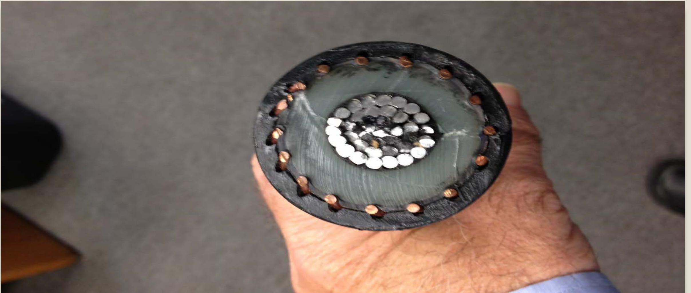
Cross-section of underground cable illustrating the aluminum core, insulator, jacket and copper grounds
