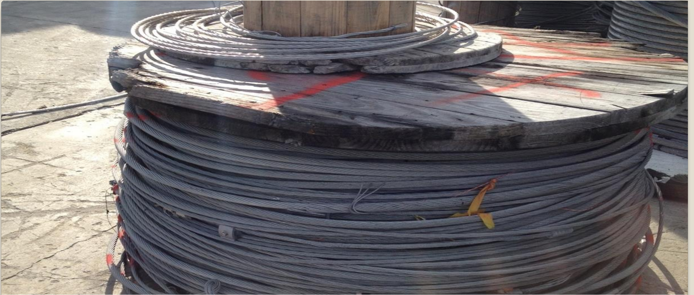
Transmission cable (ACSR) staged for processing into steel and aluminum straws
