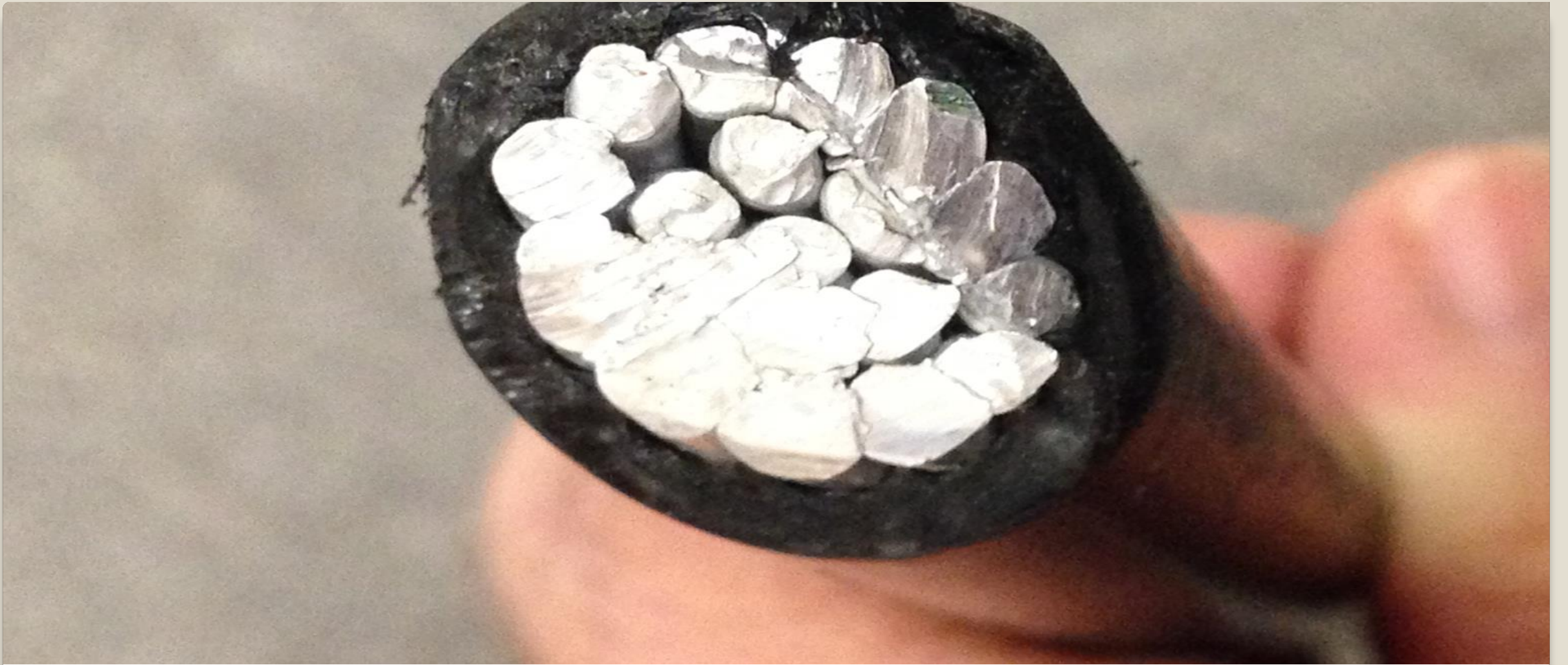
Cross-section of service wire
