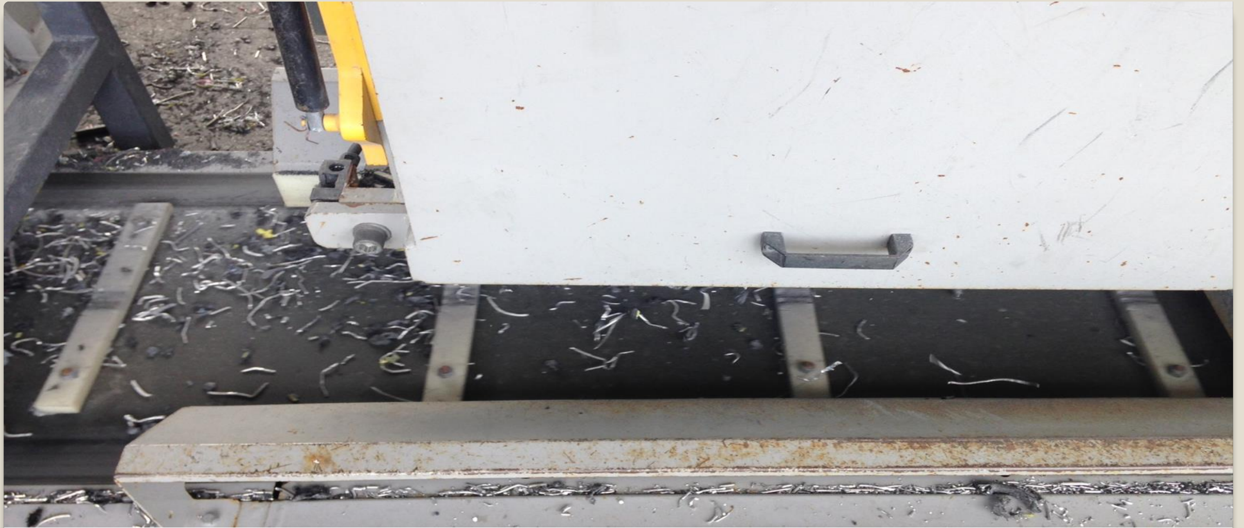
Fragmented wire and jacket after passing through shredder
