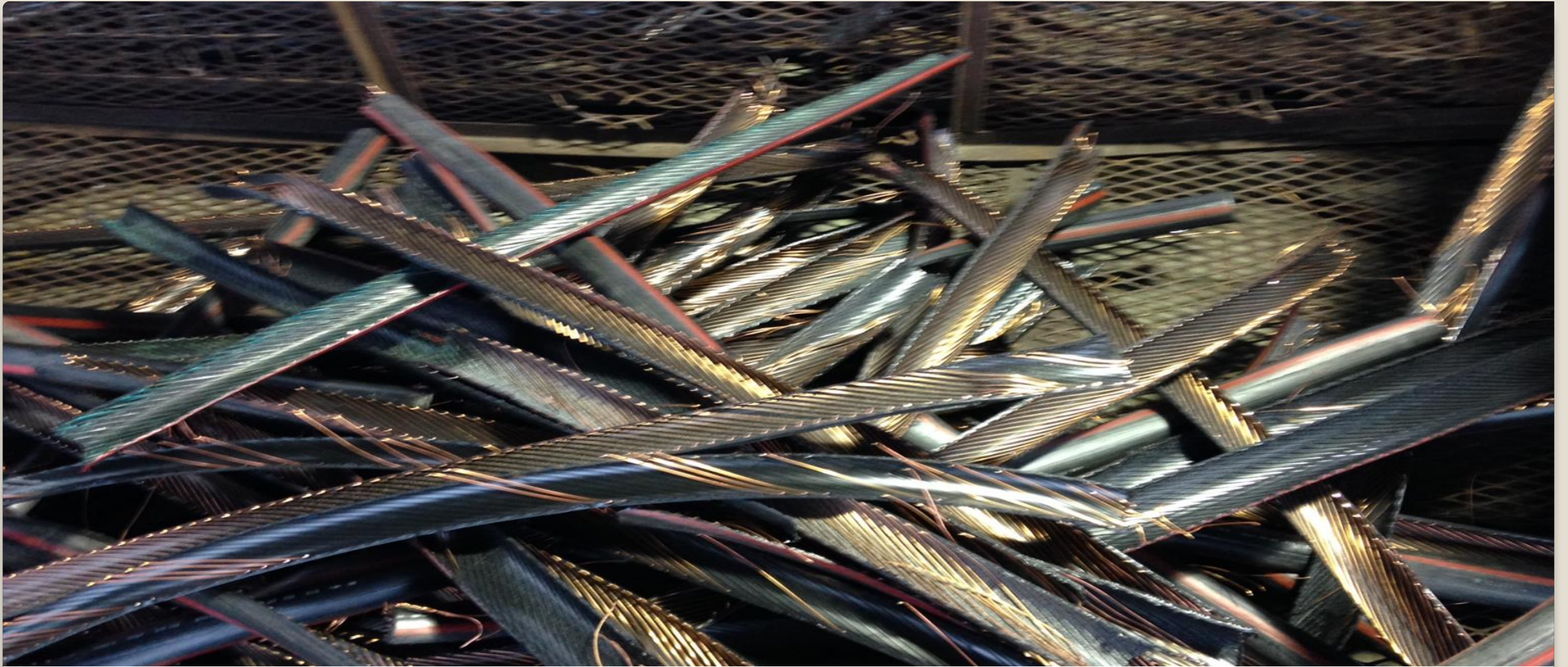
Outer jacket with copper grounds still imbedded
