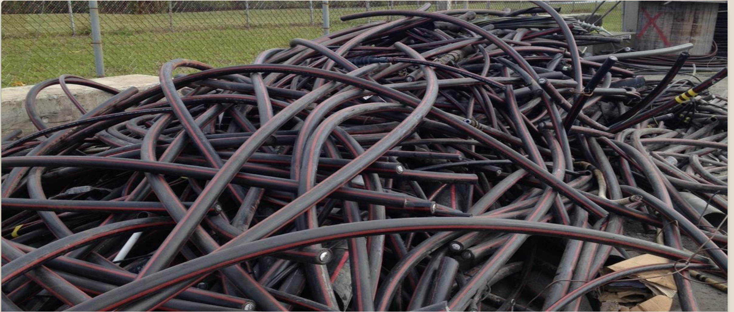
URD cable ready to be processed
